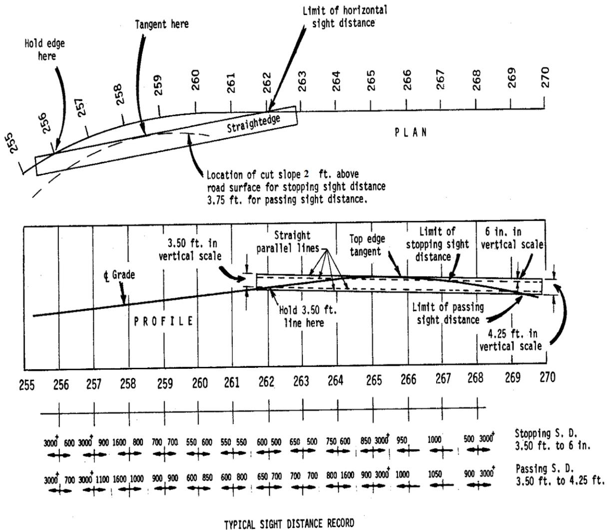
Figure 7.1—Scaling and recording sight distance on plans
