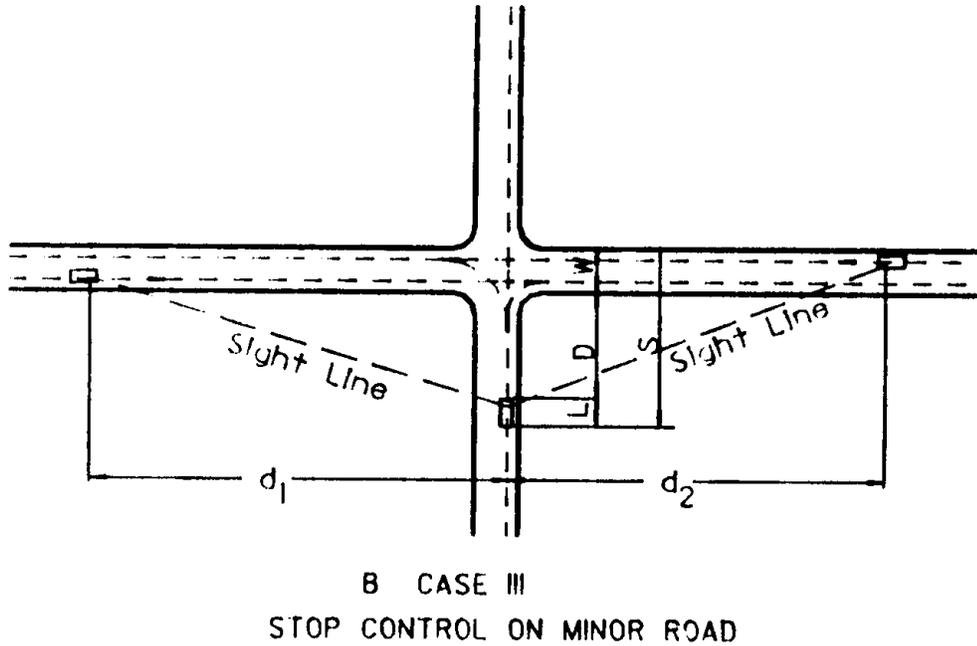
Figure 7.2—Sight distance at intersections, minimum sight triangle
