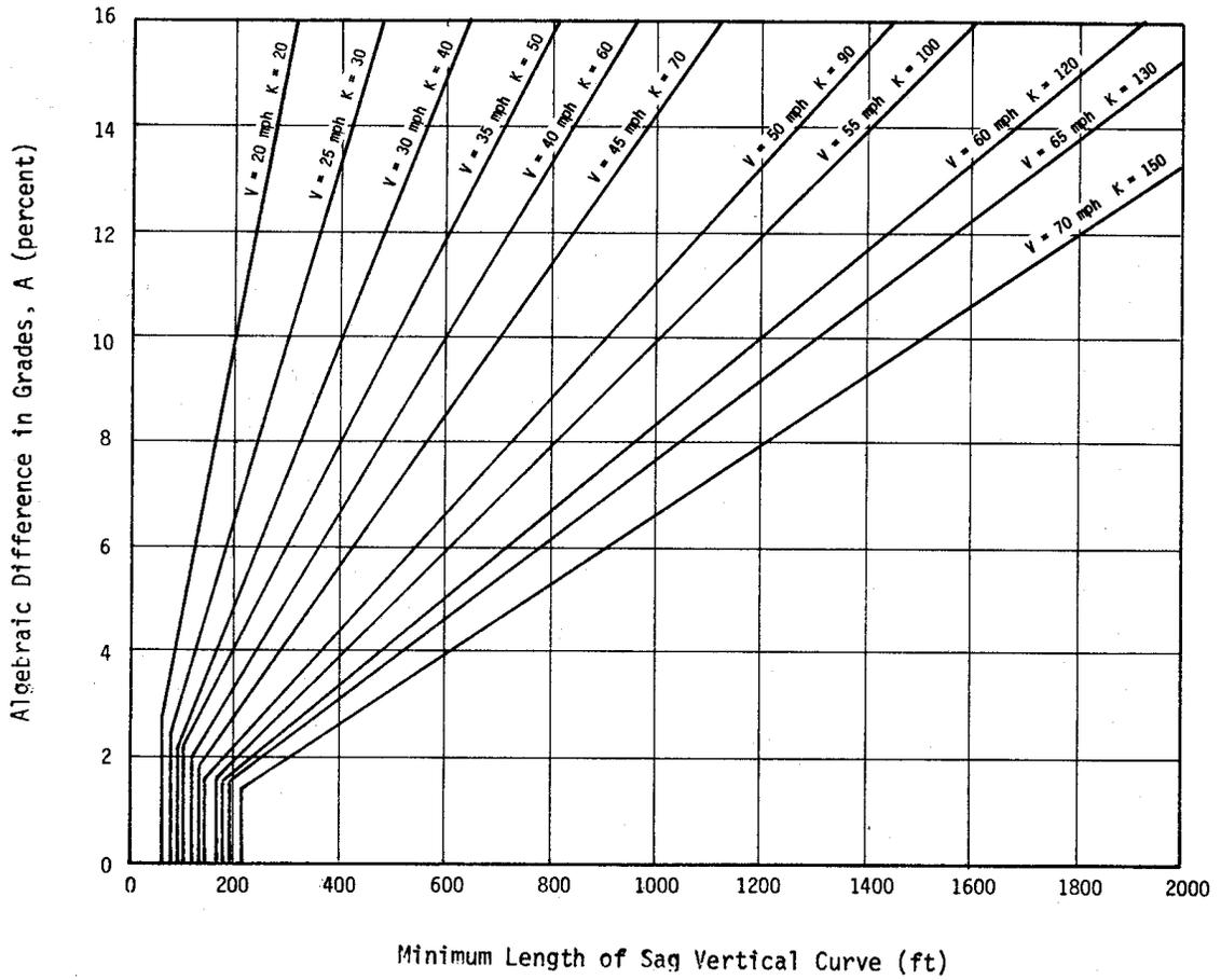
Figure 7.8—Design controls for sag vertical curves, lower range
