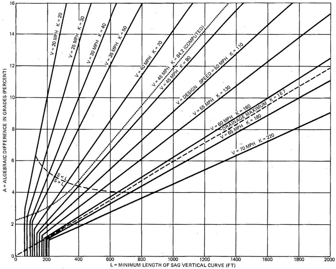
Figure 7.7—Design controls for sag vertical curves, open road conditions, upper range
