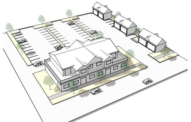
Fig. 3-27-N: Multi-family parking located behind primary structure
