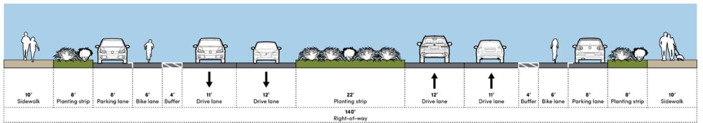
**Figure 3.4:** Rural Arterial Cross Section
