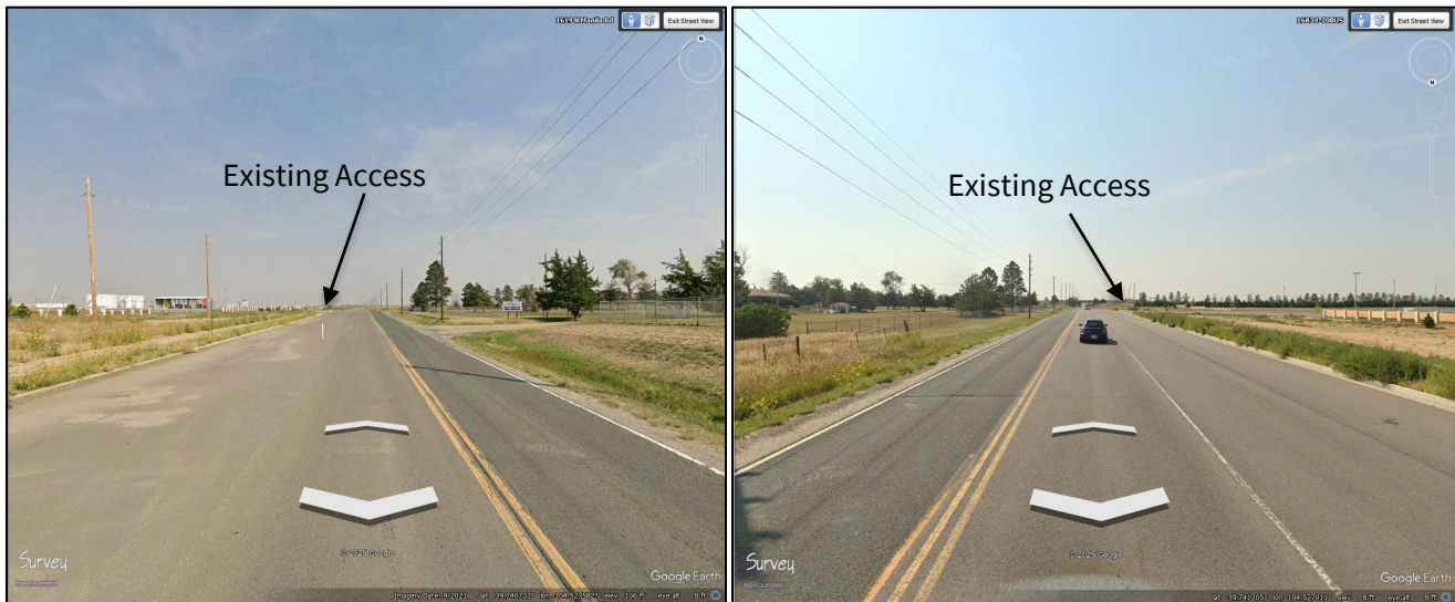
Figure 2. Sight stopping distance. Left picture 400 feet south of the existing access facing north. Right picture 400 feet north of the existing access facing south.
